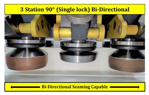
The seamer must be engaged in this manner. Failure to do so will result in panel damage.
